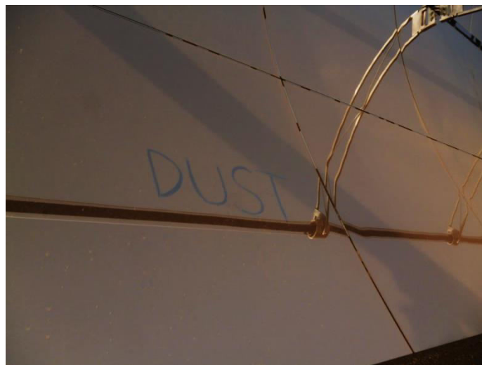
Figure 1.1. 'Dust' on a parabolic trough collector at Plataforma Solar de Almería, February 2016 (source: DLR)
